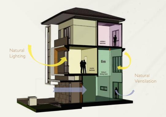
Window at both facade to maximize natural lighting to every room. Cross ventilation at living-dining room and high ceiling to bring in thermal comfort.
